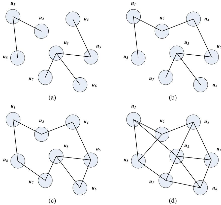
**Fig. 1.** Graph connectivity: (a) non connected, (b) 1-connected, (c) 2-connected and (c) 3-connected.
